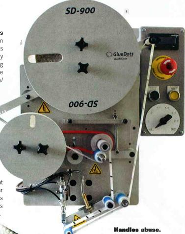
The photoelectric sensor (left) communicates with the SD-900's controller so that the movement of the roller applicator can be tightly synchronized with the speed of the conveyor carrying the object that receives the Glue Dot.
